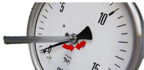
Fig. 10: Micro adjustment indicator
