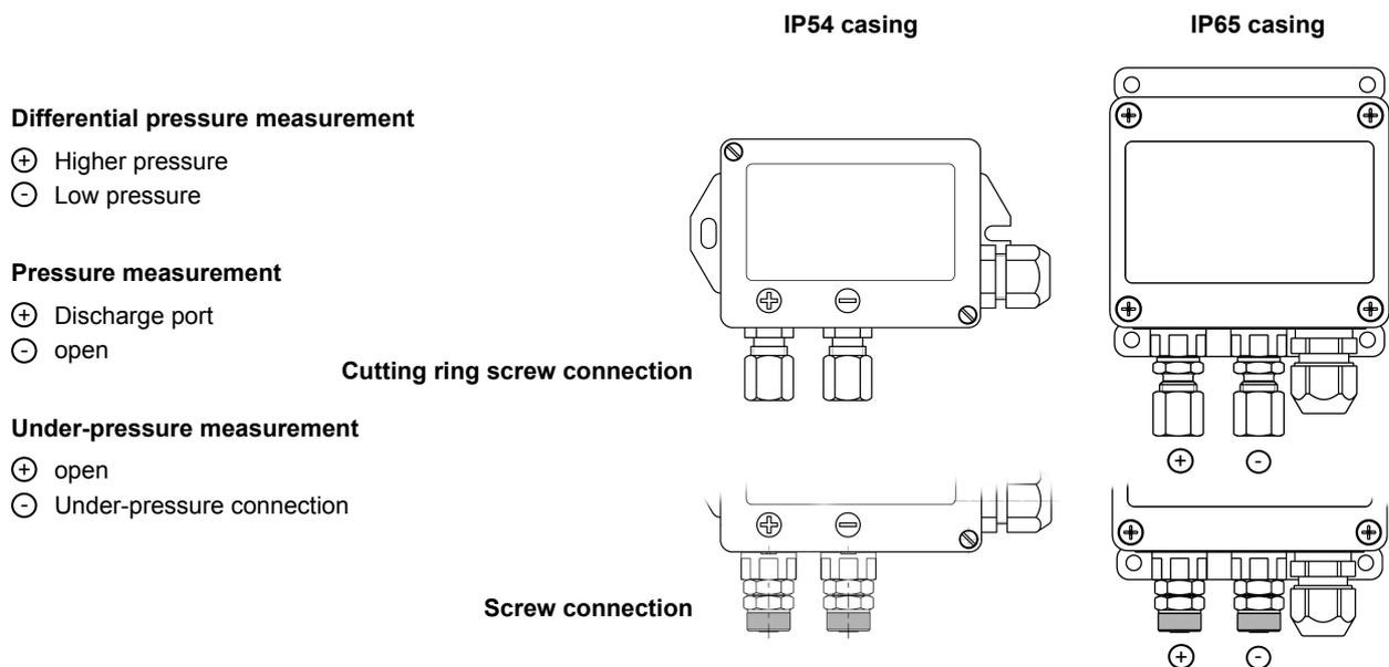
Fig. 5: Process connection
