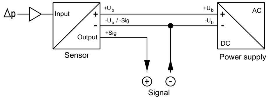
Fig. 6: 3-conductor circuit
