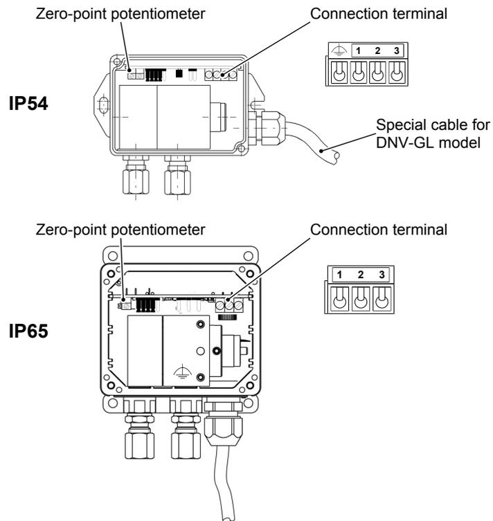
Fig. 7: Cable connection
