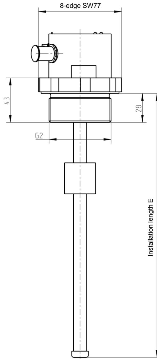
Installation length E = Probe length L + 5 mm
