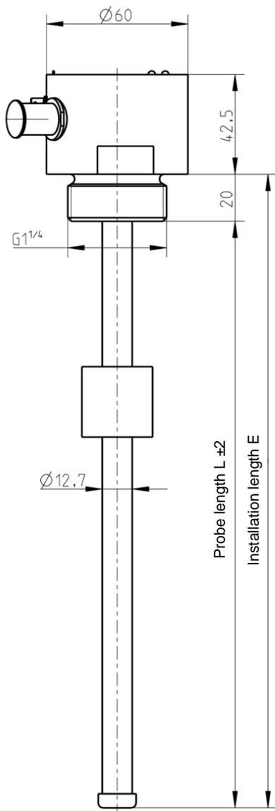
Installation length E = Probe length L + 20 mm
