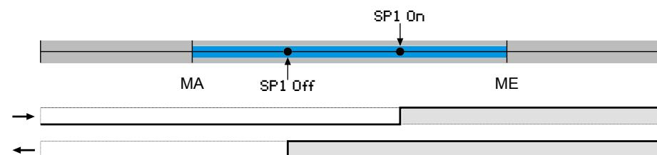
If the parameter **SP1 on < SP1 off**, the contact pulls, if the measured value lies between the parameter values:
