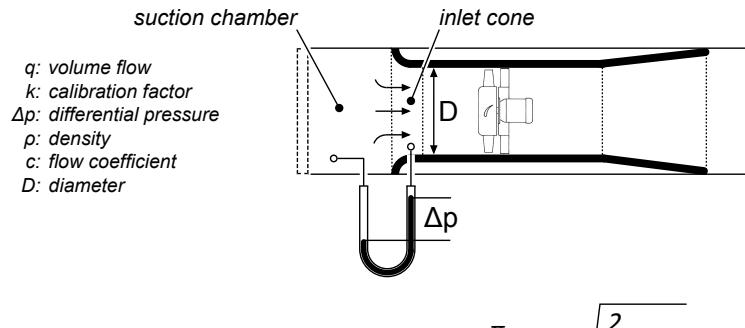
Fig. 78: Volume flow measurement
