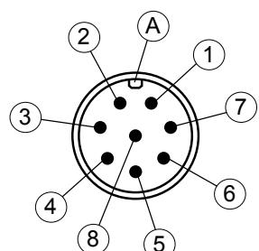
Fig. 16: M12 plug 8-pin
