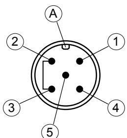
Fig. 13: M12 plug 5-pin+bridge
