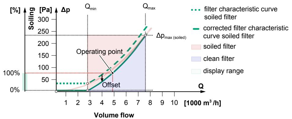
Fig. 109: Correction value square-root filter characteristic curve
