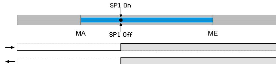
If the parameter **SP1 on > SP1 off**, the contact pulls, if the measured value exceeds the SP1 on. The contact only drops again if SP1 Off is undercut.
