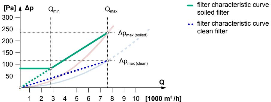
Fig. 106: Approximated linear filter characteristic curve
