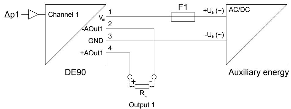
*Fig. 11: 3-conductor circuit (1 channel)*
