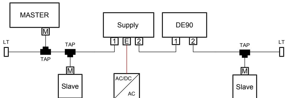
Fig. 19: Modbus connection
