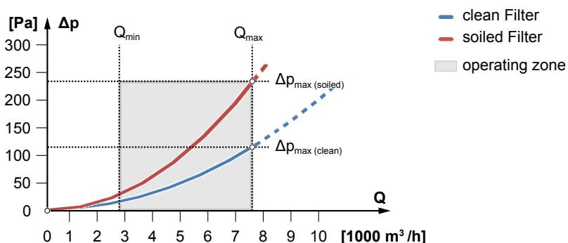
Fig. 105: filter characteristic curve
