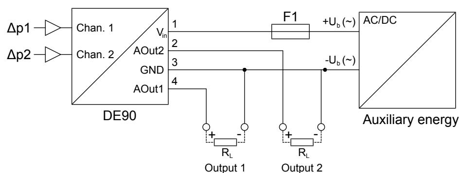
*Fig. 12: 3-conductor circuit (2 channel)*
