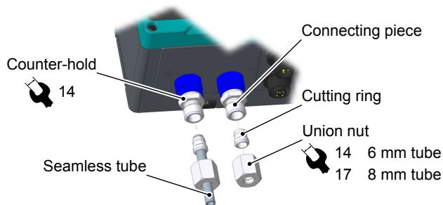
Fig. 9: Counter-hold for cutting ring screw connections
