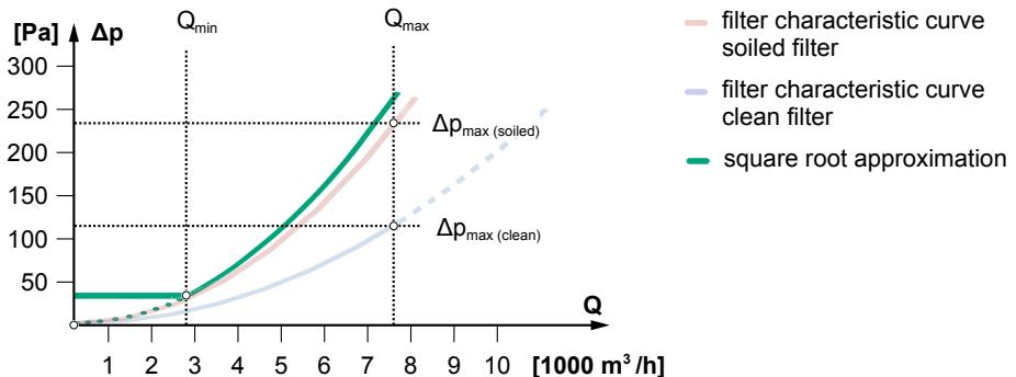
Fig. 108: Square-root approximation of the filter characteristic curve
