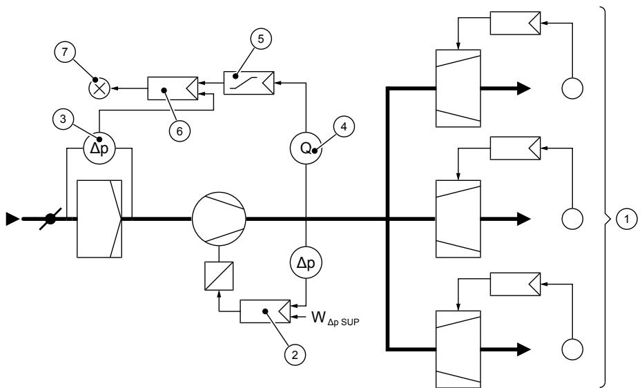
Fig. 103: Principle Diagram for Filter Monitoring
