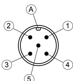
Fig. 22: M12 plug 5-pin
