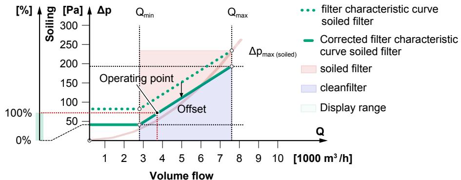
Fig. 107: Correction value Linear filter characteristic curve
