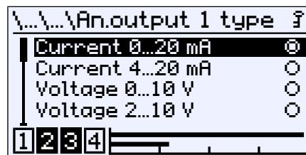
Fig. 113: Analog output 1 type
