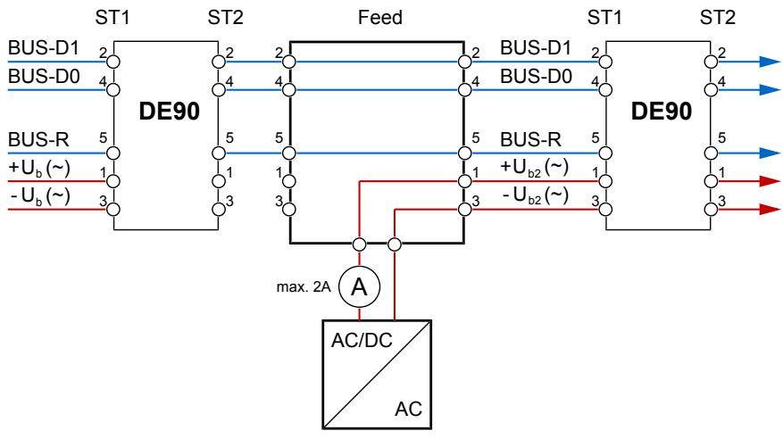
Fig. 21: Intermediate supply
