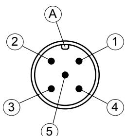
Fig. 14: M12 plug 5-pin
