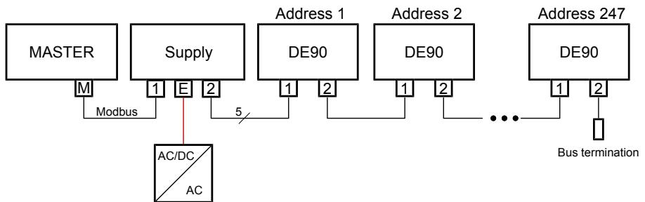
Fig. 18: Modbus RTU network
