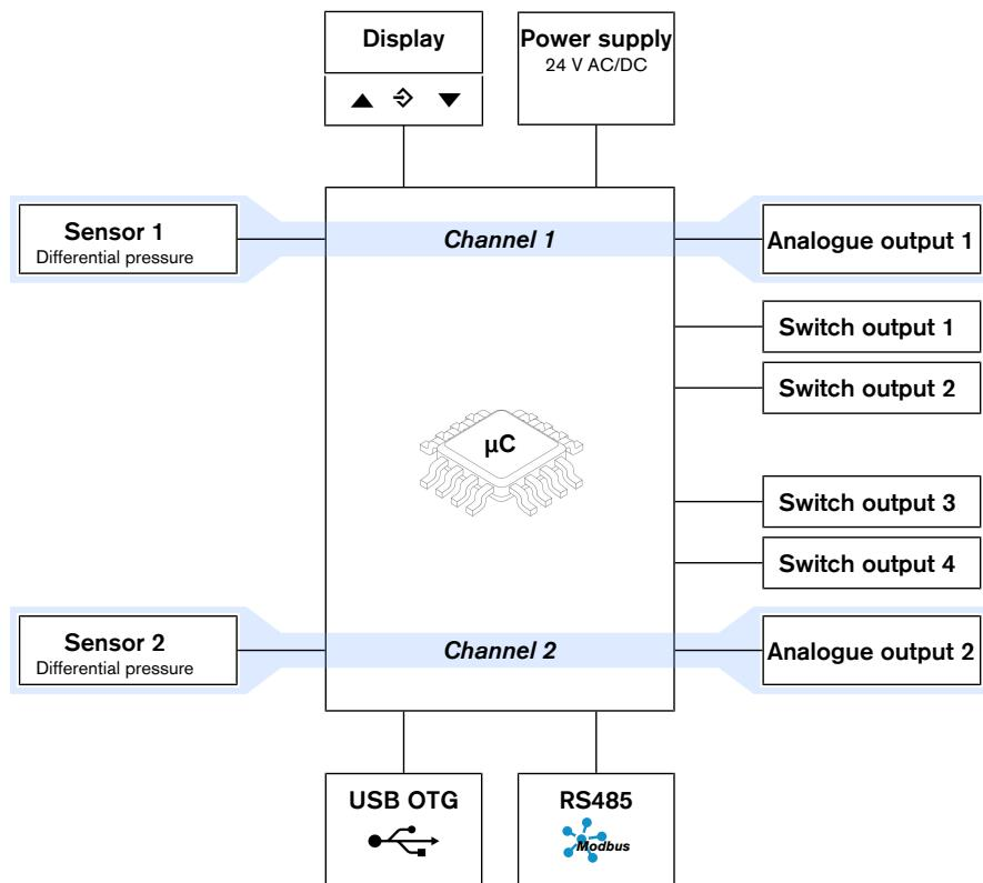
Fig. 1: Function diagram
