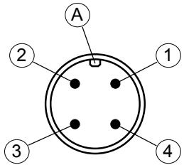
Fig. 15: M12 plug 4-pin
